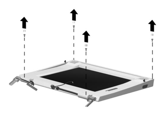
Figure 5-31. Removing the Display Bezel Screw Covers and Screws
